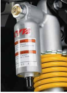
rebound and high/low speed compression adjustments. More performance oriented valving than stock vehicle. Use original stock spring. Sold in pairs.
