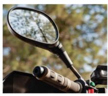
True vision surface. Matte finish. Stem includes 3/8" (10 mm) thread. Bracket (715000190) is required for installation on an Outlander without windshield.
