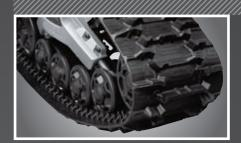
Biggest contact patch, highest ground clearance, lowest steering effort, reduced friction and vibration with heightened rubber overmold wheels.
