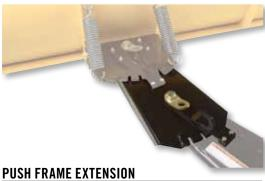
31 cm [12 ¼"] chassis extension for use with Apache Track systems. Increases angle and enables extra blade rotation. Cannot be used with Manual EZ Lift System (703500522) and Remote Angling System (715000260).
